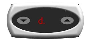
PRESSING THE INDICATED BUTTON TO INPUT A NUMBER THAT FOR THIS MACHINE WOULD HAVE THE VALUE EQUAL TO 1.6 THE VALUE WILL INCREASE BY PRESSING THE BUTTON DX AND DIMINISH BY PRESSING THE BUTTON SX
