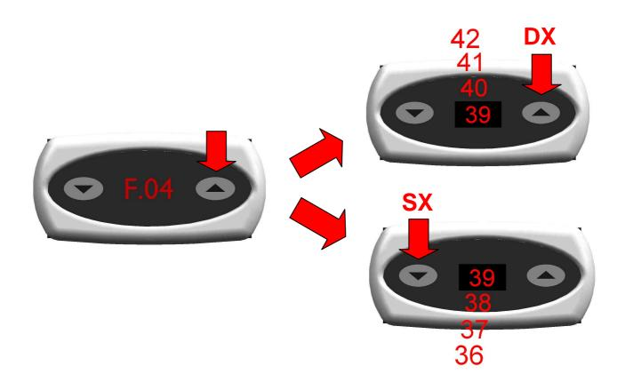
THE AMOUNT INSERTED (INCREASED OR DECREASED) REPRESENTS THE DIFFERENCE BETWEEN THE TEMPERATURE OF THE BOILER WATER AND THE WATER THAT IS EXTRACTED FROM THE GROUP HEAD.
