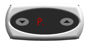
PRESSING THE INDICATED BUTTON TO INPUT A NUMBER THAT FOR THIS MACHINE WOULD HAVE THE VALUE EQUAL TO 1 THE VALUE WILL INCREASE BY PRESSING THE BUTTON DX AND DIMINISH BY PRESSING THE BUTTON SX
