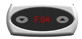
PRESSING THE INDICATED BUTTON TO INPUT A NUMBER THAT FOR THIS MACHINE WOULD HAVE THE VALUE EQUAL TO 39 THE VALUE WILL INCREASE BY PRESSING THE BUTTON DX AND DIMINISH BY PRESSING THE BUTTON SX
